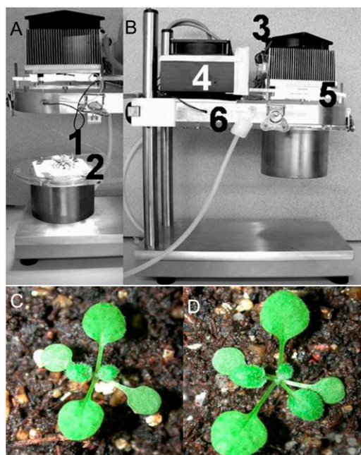
Figure 5. Pictures of an open (A) and a closed (B) Arabidopsis cuvette. Thermocouples (1) inside of the cuvette measure leaf temperature continuously. In the basement of the cuvette system, the Arabidopsis rosette is fixed and the soil is covered with plastic pieces (2). Ventilators and a cooling element (3) cool down the LED light head (5) and the Peltier element (4). The inlet air port (6) is placed on the opposite of the outlet air port. Shown are pictures of wild-type (C) and transgenic (D) Arabidopsis plants at the age of 2 weeks.
