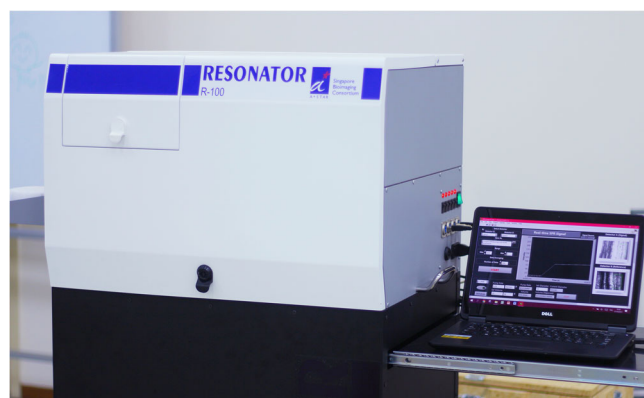
FIGURE 2 Device prototype of the surface plasmon resonance imaging biosensor
