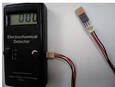
FIGURE 13 Portable microneedle-based electrochemical sensor for detection of hydrogen peroxide levels
