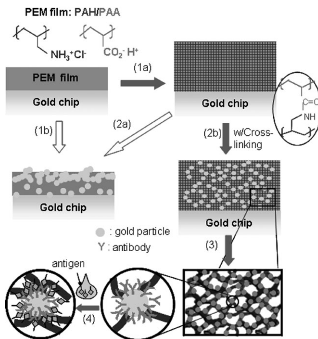
Scheme 1. The procedure used to create a gold nanoparticle-hybridized polymer film on a biosensor chip: (1a) pore formation; (2b) gold nanoparticle synthesis in porous film after crosslinking of the film; (3) antibody immobilization; (4) antigen detection. Note, a gold synthesis without crosslinking of the porous film, process (2a), produces the same result obtained from non-porous film (1b). The total processes to create a functional SPR coating follow the filled arrows.
