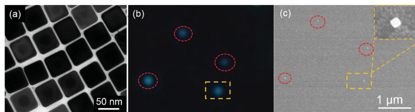
Figure 2. a) TEM images of Au@Ag NCs. b) DFM image of the Au@Ag NCs on an ITO glass slide. c) In situ SEM image of the selected area Au@Ag NCs in DFM image (insert: the enlarged SEM image).
