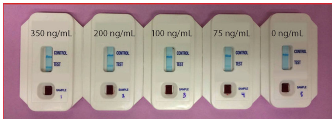
Fig. 7 Whole-blood lateral flow assay at spiked myoglobin concentrations ranging from 350 ng/mL ( left ) to 0 ng/mL. 50 \mu L blood samples were spiked with various myoglobin concentrations and added to 50 \mu L of an antibody/liposome solution. This mixture was gently vortexed, and after 5 min, all 100 \mu L were added to the sample pad. Results were observed after 15 min. A visible signal at the test line could be seen at a spiked myoglobin concentration of 75 ng/mL (see Notes 8 and 9 )
