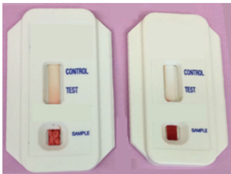
Fig. 4 Whole blood applied to lateral flow assay membranes assembled in injection molded housings to test sample pad types. No test or control lines were immobilized. Significant hemolysis was observed in the left assembly which yielded a pink colored background which could potentially obscure weak signals, whereas a clear background was available in the right assembly
