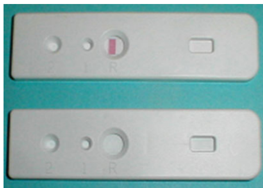
Fig. 3 Lateral flow assay membranes assembled in injection molded housings. In the presence of the target analyte, a sandwich complex forms with dye-encapsulating liposomes resulting in a magenta-colored band at the capture zone that is proportional to target concentration ( top ). In the absence of target analyte, no band is visible as no sandwich complex has formed ( bottom ). Though not necessary, these LFA membranes were housed in more user friendly packaging using a plastic cassette made using injection molding and designed for addition of liposome/target mixture in hole #1 and addition of running buffer in hole #2. Readings can be taken in the “R” hole
