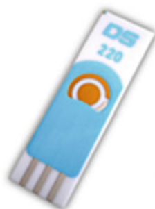
Fig. 5 Au screen-printed electrode (DropSens ref. DRP-220)
