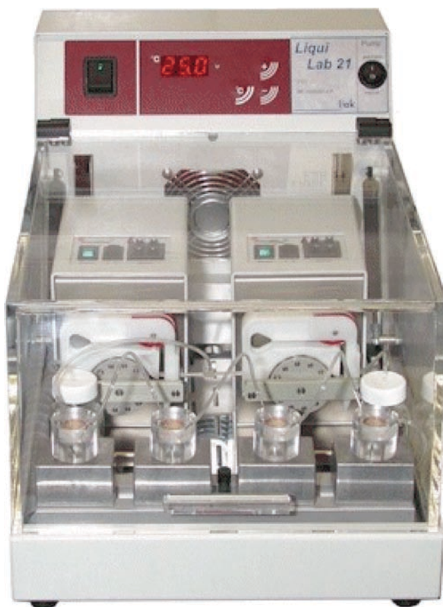
Fig. 4. The QCM biosensor device used for this study. Four flow chamber systems, each connected to an oscillator, are combined within a peristaltic pump flow system and inserted into a thermostatic device. Data were collected and evaluated by a computerized system
