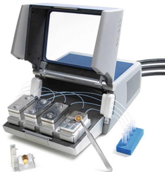
Fig. 4 The Q-Sense E4 system, showing four flow cells in a temperature-control chamber. The right-hand flow cell is open and a gold-coated quartz crystal chip is shown held in a pair of tweezers, ready for placement onto the “o”-ring-sealed flow chamber (reproduced from Q-Sense E4 manual)
