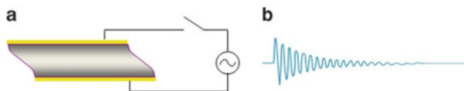
Fig. 1 (a) Cross-sectional representation of the strain of a quartz crystal driven by an alternating electric current when the circuit is closed. (b) Decaying resonant frequency when the circuit is opened
