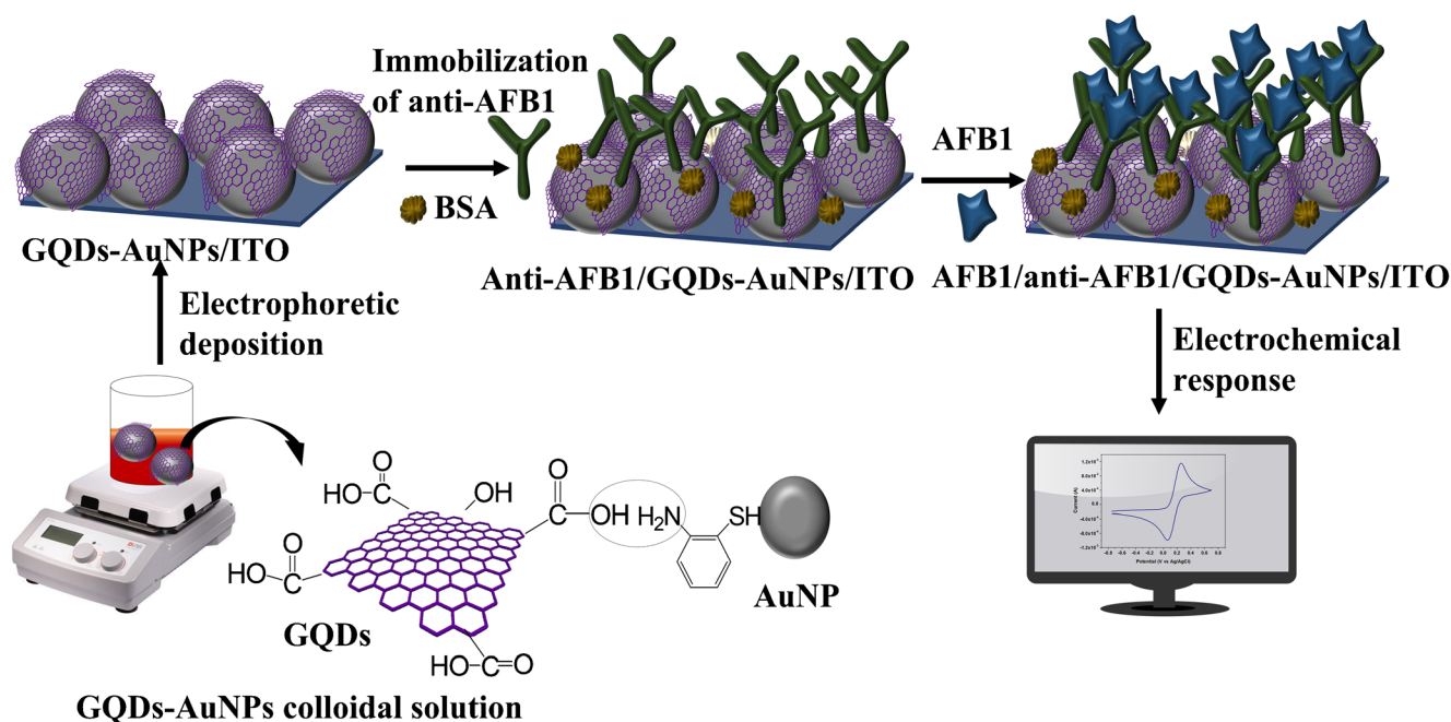
Fig. 1 Schematic representation of the synthesis of composite graphene quantum dots-gold nanoparticles (GQDs-AuNPs) and Electrochromatic Deposition (EPD) of synthesized composite onto ITO electrode and
