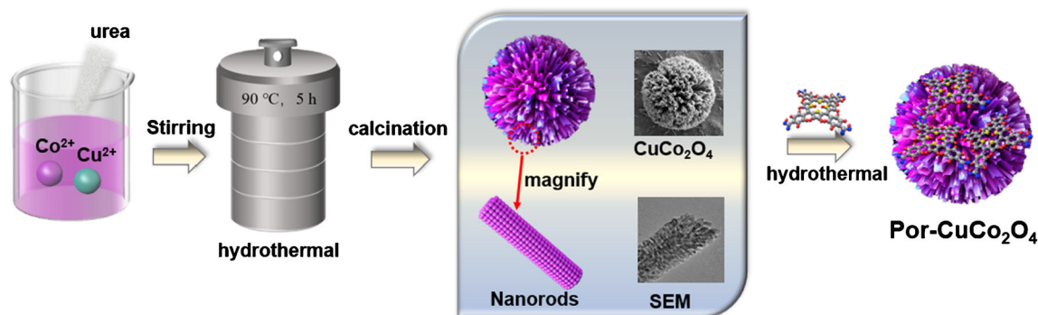
Scheme 1 Schematic illustration for the formation process of urchin-like \text{Por-CuCo}_2\text{O}_4 nanospheres
