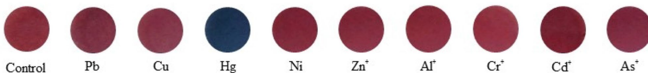
Fig. 8 The cropped digital image of brn-AuNPs with different heavy metals after colorimetry reaction
