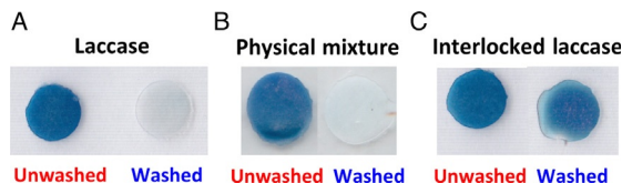
Fig. 8 Synthesis validation for (C) nanoarmored laccase interlocked with paper fibers. All samples were washed to remove any unbound material. Controls are (A) adsorbed laccase and (B) laccase physical mixtures (unpublished work).
