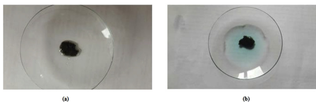
Fig. 17. Interaction with enzyme-immobilized nanofiber to substrate. (a) nanofiber not interacted with substrate (b) nanofiber interacting with substrate.
