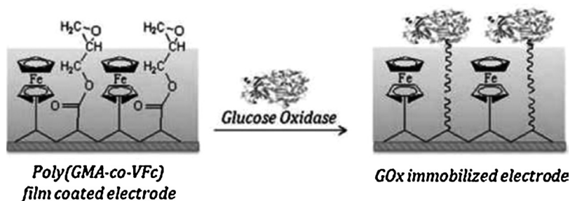
Fig. 4. Immobilization of enzyme onto a polyGMA-co-VFc film electrode, reprinted with permission of Ref. [92].
