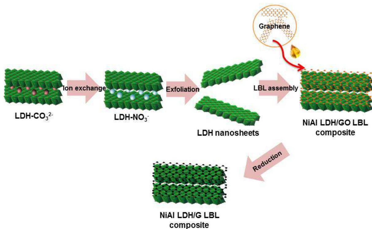
Fig. 1. Flow chart presentation of different steps involved in the fabrication mechanism of NiAl LDH/G LBL nanocomposites.
