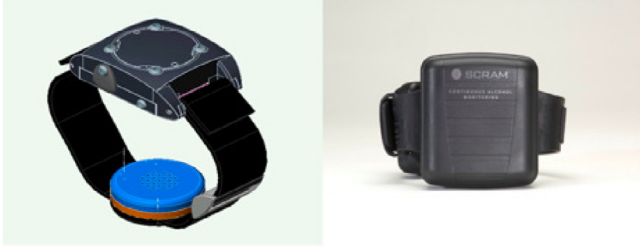
Fig. 1. Left: The WRISTAS™7 transdermal alcohol biosensor. Right: The Alcohol Monitoring System (AMS) Secure Continuous Alcohol Monitoring (SCRAM) system.
