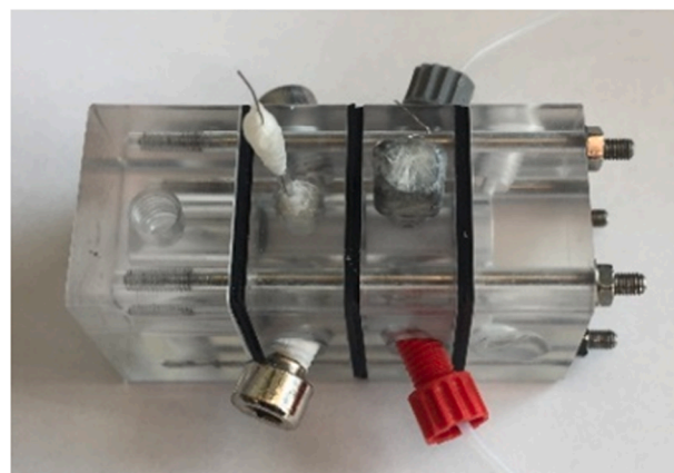
Fig. 5. Photograph of the flow-through cell. A schematic illustration can be found in the supporting information (Fig. S1).
