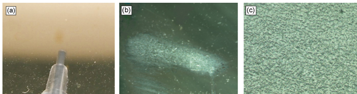
Fig. 2. (a) Photograph showing polymer spot on the gold-coated SPR slide, clearly visible with the naked eye, the width of the pencil lead is 0.5 mm. (b) Optical micrograph of a polymer spot, similar to that shown in (a). The spot is approximately 2 mm \times 0.5 mm in size. (c) Close-up of the surface of the same polymer spot at 40 \times higher magnification.
