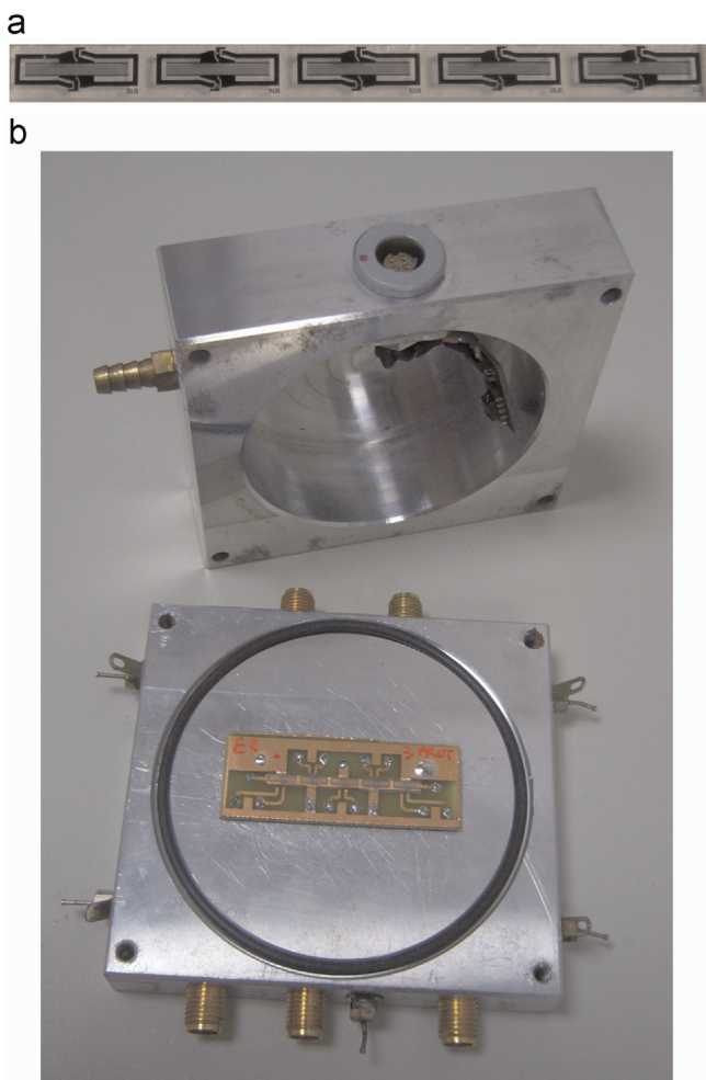
Fig. 1. Photo of the bio-electronic nose system: (a) array of SAW resonators; (b) bio-nose system with measurement chamber and conditioning electronics.
