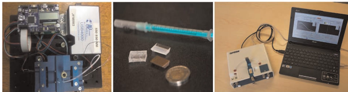
Fig. 1. (Left) Picture of the electronics and optics of the prototype system. Dimensions: 181 (L)×166 (w)×55 (H) mm 3 . Weight: 1.3 kg. (Middle) Picture of a gold-coated Dove prism and PDMS fluidic cell. A Canadian 2$ coin and a 1 mL syringe show the scale. (Right) The SPR system is controlled by a 9" laptop and requires no external power supply.
