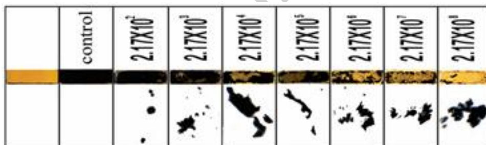
Figure 1: a) Colorimetric Listeria monocytogenes protease sensor probe using D-amino acid covalently bound to a magnetic nanobead; a) before adding the sample to the specific Listeria monocytogenes protease substrate; b) after adding different concentrations of Listeria monocytogenes protease solutions.
