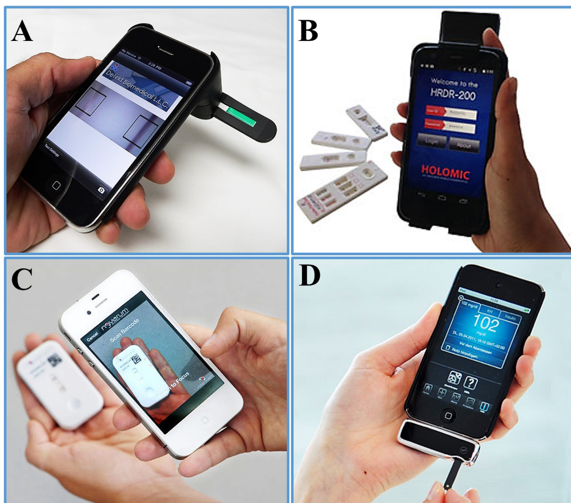
Fig. 2. Commercial readout devices (A) iPhone rapid diagnostic lateral flow reader. Courtesy of Detekt Biomedical L.L.C. (B) Android-based lateral flow reader. Courtesy of Holomic L.L.C. (C) Novarum reader. Courtesy of British Biocell International. (D) iBG star. Courtesy of Sanofi.
