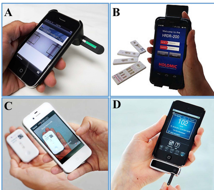
Fig. 7. Commercial readout devices; (A) iPhone rapid diagnostic lateral flow reader. (B) Android-based lateral flow reader. (C) Novarum reader. (D) iBGStar. Reproduced with permission from (Syedmoradi et al., 2017) Copyright 2017 Elsevier B.V.
