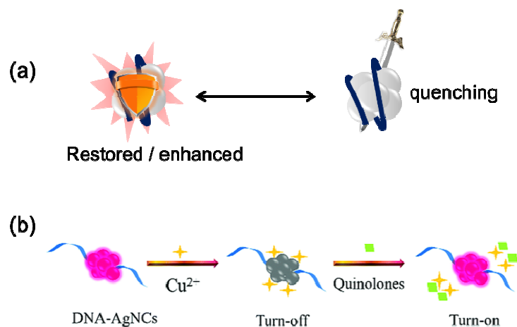
Figure 2. (a) Schematic depiction of the LFP-DAGNCs based on direct interaction. (b) Illustration for the detection of quinolones based on DNA-AgNCs– \text{Cu}^{2+} system. (Copyright © The Royal Society of Chemistry 2018)
