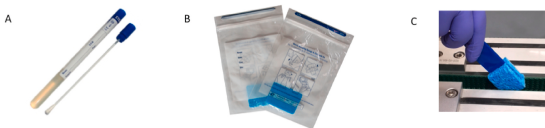
Fig. 1. Different swab types commercially available for environmental and hygiene swabbing. A: Cotton tip swab; B: Carcass sampling sponge; C: EnviroStik (sponge with breakpoint handle).
