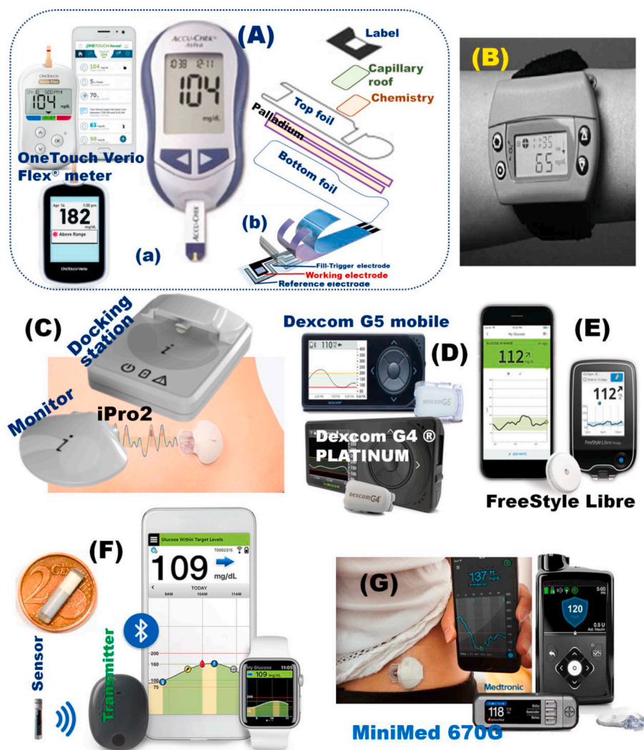
Scheme 14. The schematic design shows an overview of CGM's current commercial devices for CGM including (A) a glucometer for blood glucose sensor [Yetisen et al., 2014], (Emran et al., 2020b)] Copyright © 2018–2020 LifeScan IP Holdings, LLC. (a) Commercial Products and (b) the composition of a test strip; (B) GlucoWatch® biographer [Tierney et al., 2001]] Copyright © 2001 Elsevier Science B.V.; (C) iPro2 sensing system contains monitor and docking station [ ( https://www.mesm.com/prod/ )] Copyright©N avantor®; (D) Dexcom G4® PLATINUM ( https://www.diabetesnet.c ) Copyright © https://www.diabetesnet.com/ ; (E) FreeStyle Libre continuous glucose monitor [ (Schierenbeck et al., 2017)] Copyright © 2016 Diabetes Technology Society; (F) the Eversense System [ ( https://global.eversensed )], and (G) the Medtronic 670G device ( https://www.diabetesdaily , 2018) Copyright © 2005–2021 Thrivable Inc. All rights reserved.
