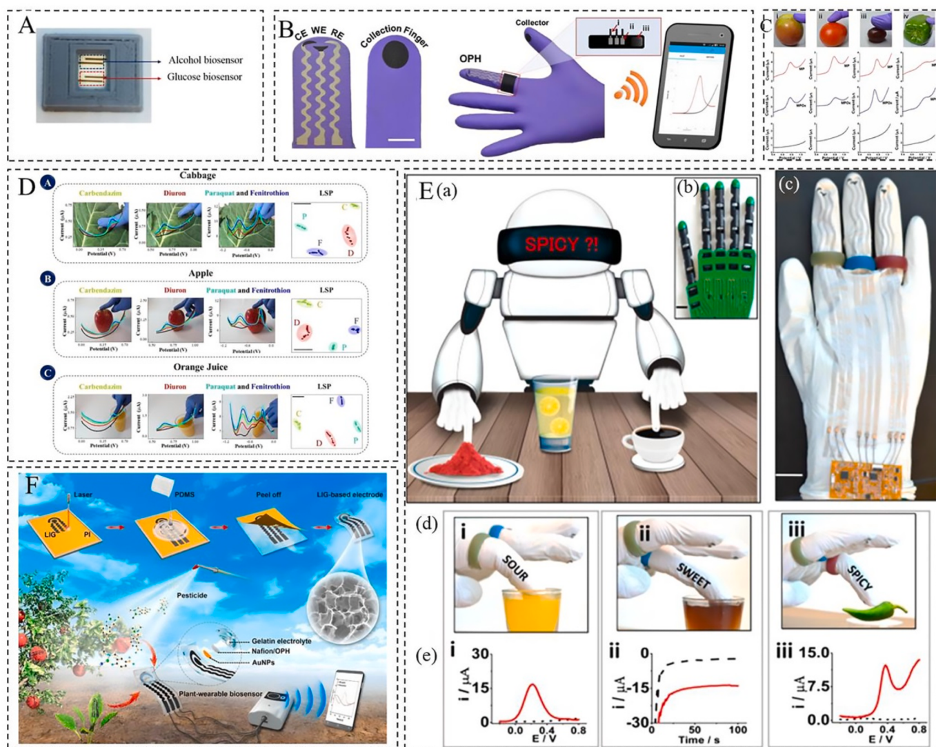
Fig. 7. (A) Picture of a combined biosensor. (B) Flexible glove biosensor. (C) Sampling and detecting OP pesticides on the surfaces of different fruits and vegetables. (D) Photos of actual measuring conditions of wearable glove-embedded sensors on food samples. (E) Robotic sense fingers: schematics, fabrication, and analytical performance. (a) Schematics of robotic finger immersed in lemon juice, coffee, and chili powder placed on a table for the subsequent detection of sourness, caffeine, and spiciness, respectively. (b) Image illustrating the robotic hand used to develop the glove-based sense fingers. (c) Prototype of the screen-printed robotic sense fingers with long connections to the wrist where the electronic interface is located. Robotic fingers are identified with colored rings: green for carbon-printed sour fingers; blue for GOx Prussian blue-printed sweet fingers; and red for carbon-printed spicy fingers. Scale bar, 5 cm. (d) Images and (e) corresponding electrochemical data of (i) robotic sour finger dipped in orange juice and the square wave voltammetry (SWV) signature of ascorbic acid, (ii) robotic sweet finger in cherry juice and amperometry data of glucose, and (iii) spicy finger on green pepper and SWV feedback response to the presence of capsaicin. Dotted lines correspond to the blank PBS response. (F) Schematic diagram of the fabrication process of the plant-wearable biosensor based on 3D porous laser-induced graphene (LIG) and the application of in situ pesticide analysis for agricultural products.
