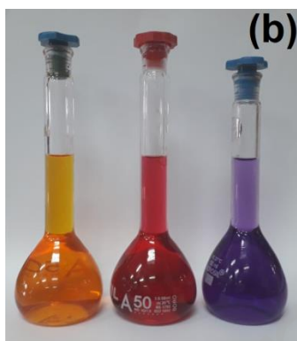
Figure 2: (a) pH correlated UV-Vis absorption spectra, and (b) color shift from orange, red to purple upon changing pH between 6.55 (Orange; pH1 at 475 nm), 6.75 (pH2 at 485 nm), 6.95 (Red; pH3 at 505 nm), 7.05 (pH4 at 505 nm), and 7.15 (Purple; pH5 at 530 nm) respectively; of TCFH 4 in acetone solution ( ca. 1.7 \times 10^{-5} \text{ mol L}^{-1} )
