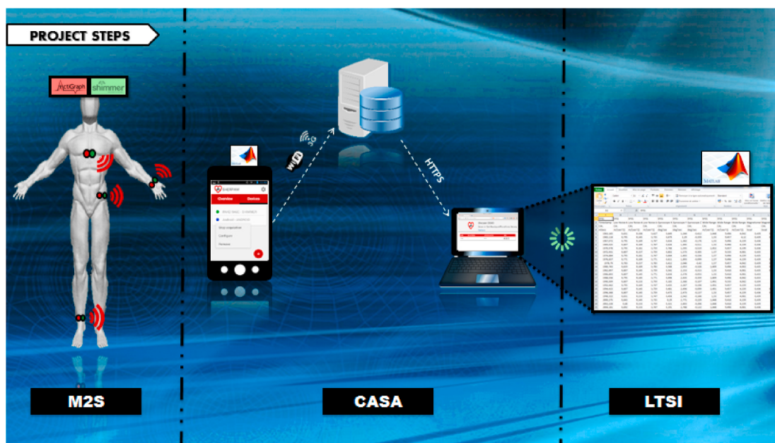
Fig. 1. Different stages for health monitoring using Sherpam system.
