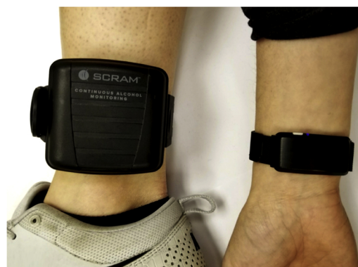
Fig. 1. AMS SCRAM ankle bracelet (left) and BACtrack Skyn wrist monitor (right) displayed side-by-side. The approximate weights of the devices are 6oz (SCRAM) and 1oz (Skyn prototype).
