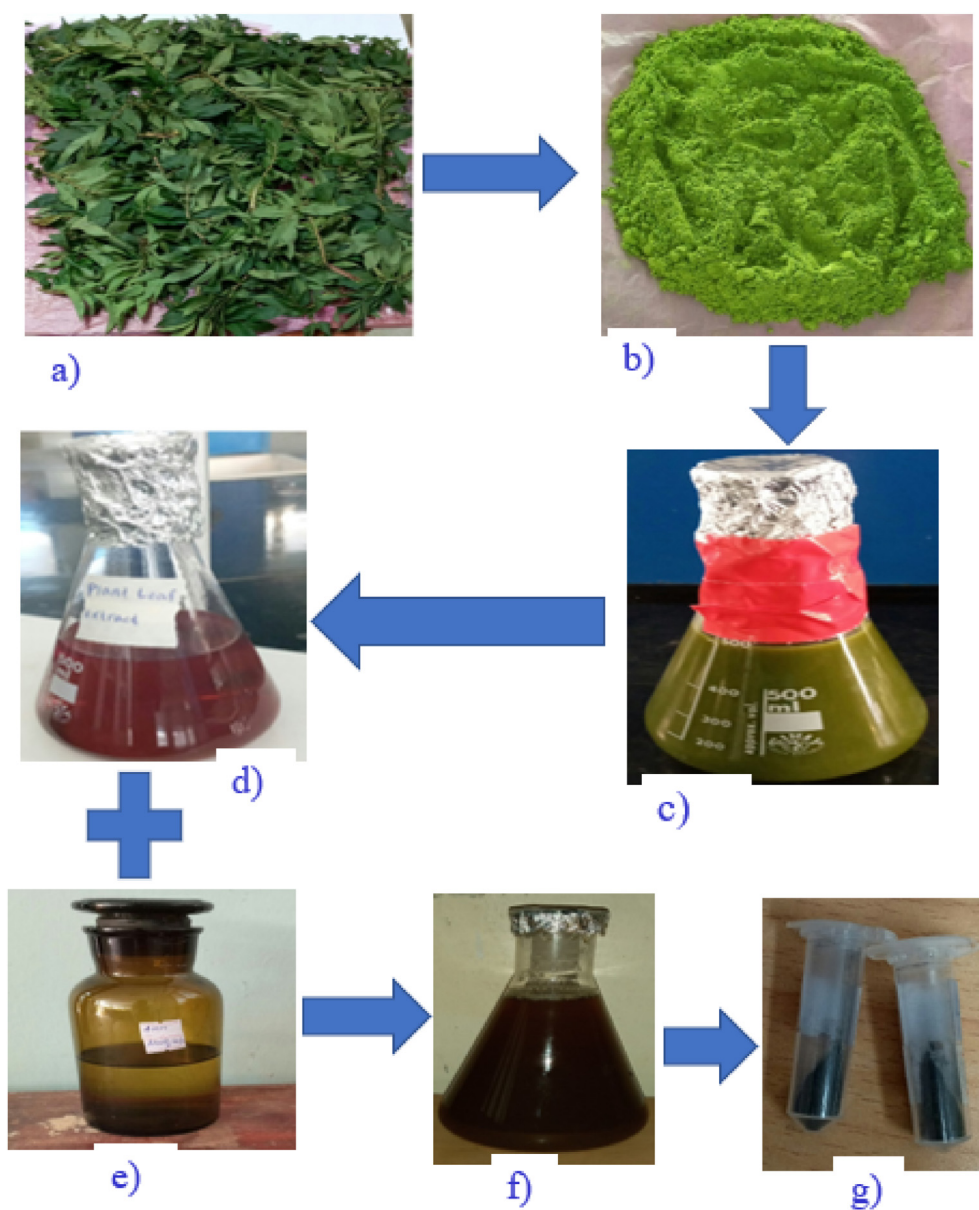
Figure 3. Green synthesis of AgNPs from HAPLE after incubation at 40 °C for 90 min, and colour change observation: a) Hagenia abyssinica plant leaf; b) Hagenia abyssinica plant leaf powder; c) Macerated Hagenia abyssinica aqueous plant leaf extract before filtration; d) Hagenia abyssinica aqueous plant leaf extract after filtration (dark-red); e) 4 mM aqueous \text{AgNO}_3 solution; (colorless); f) Colloidal AgNPs (dark-brown) and g) Powdered AgNPs.
