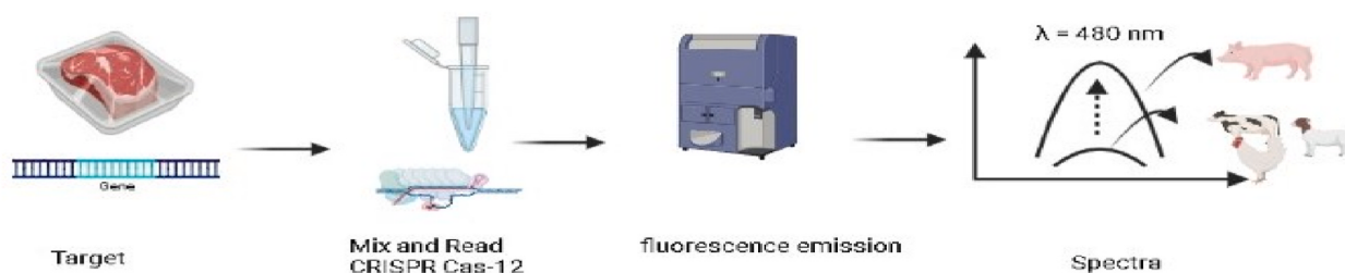
Fig. 3. The working principle illustration of halal food authentication via CRISPR-Cas12-based nucleic acid test.
