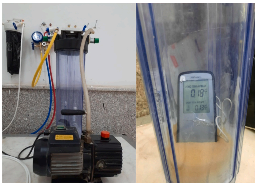
Fig. 2. a. Radon and lead detection system, b. Chamber with biosensor cell, canary device, and thermometer.
