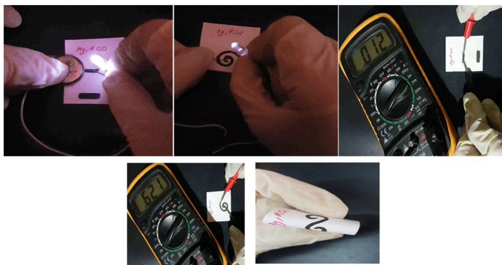
Fig. 1. Photographic images of various patterns with different thicknesses and shapes obtained by Ag/RGO nano-ink on photo paper.
