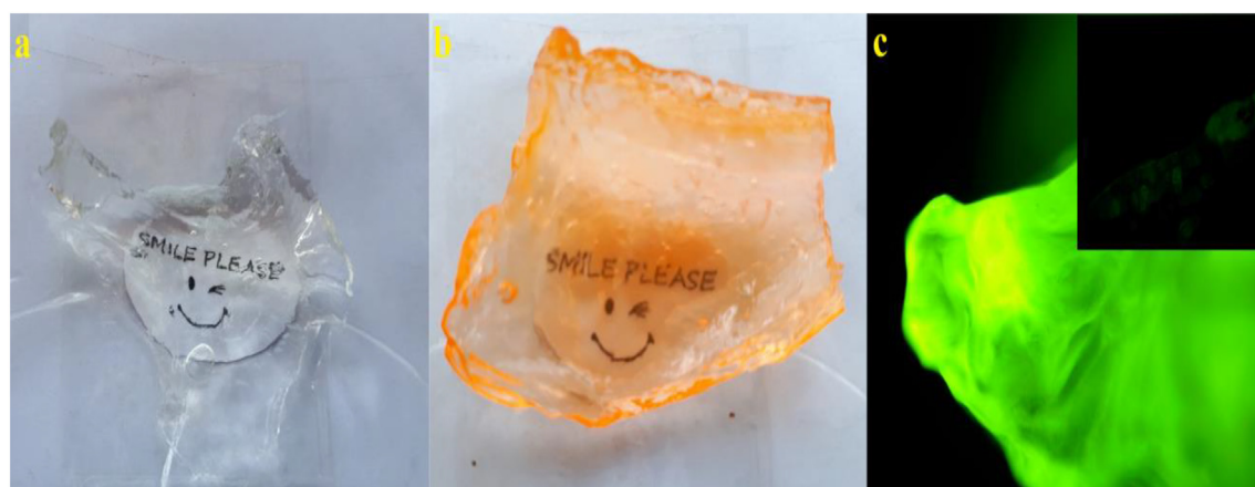
Fig. 1. For the transparency confirmation, photos of nanohydrogel were taken without QDs (a) and with encapsulated QDs (b). Photo was taken by the fluorescence microscopy of the nanohydrogel containing QDs (c), the inset shows the photo of the same sample after addition H_2O_2 .
