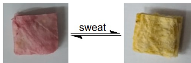
Fig. 2. Colorimetric shift of biochromic aerogel biosensor from pink to greenish-yellow upon exposure to sweat mimic solution (pH >7). (For interpretation of the references to color in this figure legend, the reader is referred to the web version of this article.)
