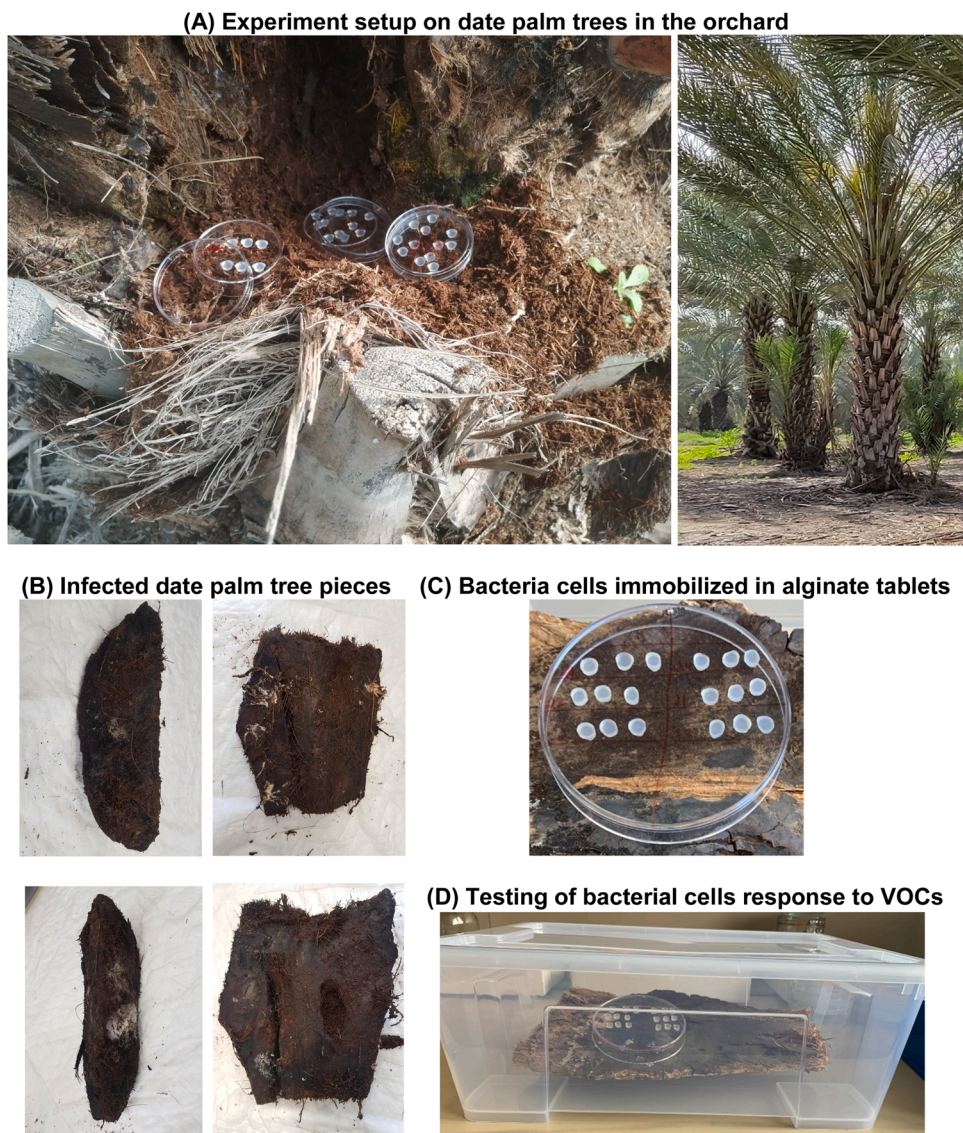
Fig. 3. Image of the experiment setup. (A) The immobilized bacteria cells were exposed to the air near infected by red palm weevil (RPW), Rhynchophorus ferrugineus , or uninfected date palm trees in the orchard. (B) Image of infected palm tree pieces collected from infested date palm trees. (C) Bacteria cells immobilized in alginate tablets. (D) Testing of bacterial cells response to VOCs in a closed container. The bacterial tablets were then placed into a 96-well microtiter plate for the measurement of their bioluminescent signal with a commercial plate reader.
