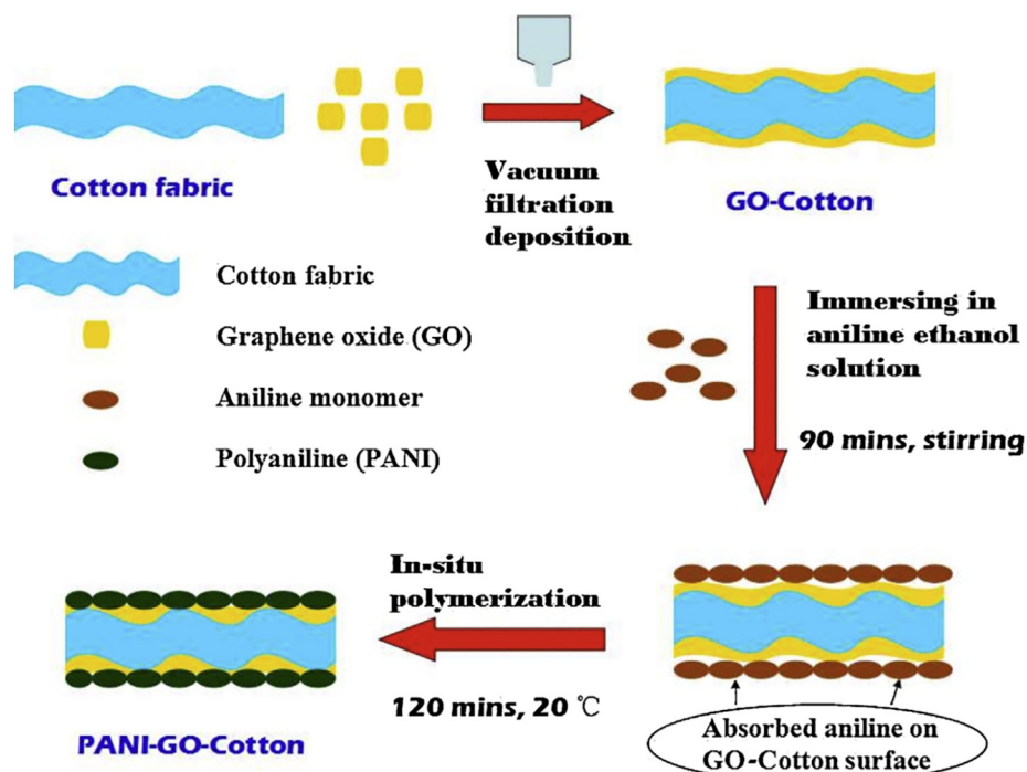
Fig. 3. Preparation procedure of PANI-GO-cotton fabric [34]. Reprinted with permission from Elsevier.
