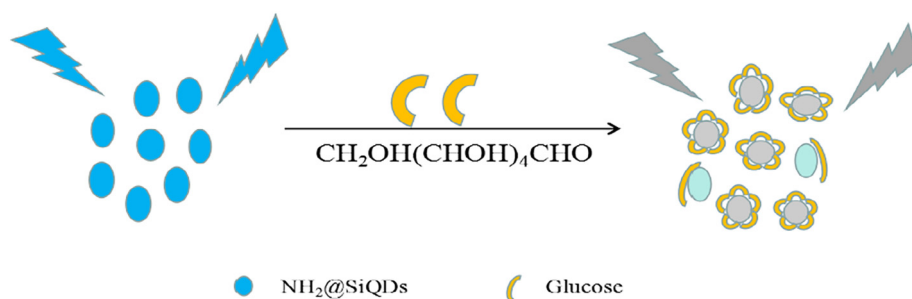
Scheme 2. Schematic illustration of the free-enzyme biosensor for sensitive glucose detection.
