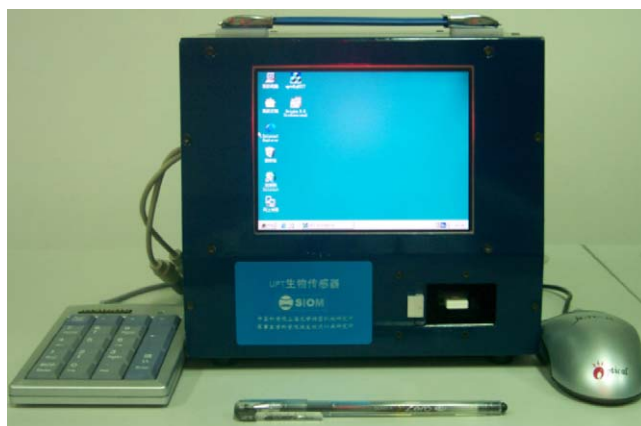
Fig. 2. Photograph of the portable prototype UPT-based biosensor.
