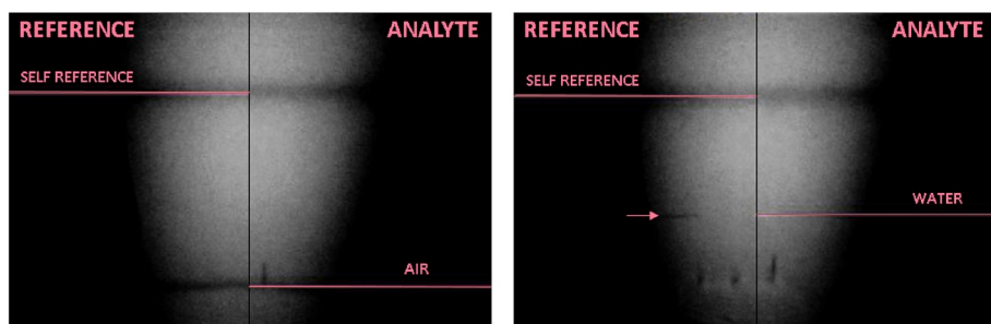
Fig. 5. Self-Referenced Silicon Dioxide Plasmonic Chip. The self-referenced plasmon waveguide resonance (SPRWR) SiO 2 chip allows for a stable self-reference measurement due to its multi-layered structure of: 420 nm SiO 2 - 40 nm Ag - 480 nm SiO 2 , thus minimising the sample volume required. The top dark line is the self-reference line while the bottom dark line corresponds to the PWR mode. (For interpretation of the references to color in this figure legend, the reader is referred to the Web version of this article.)
