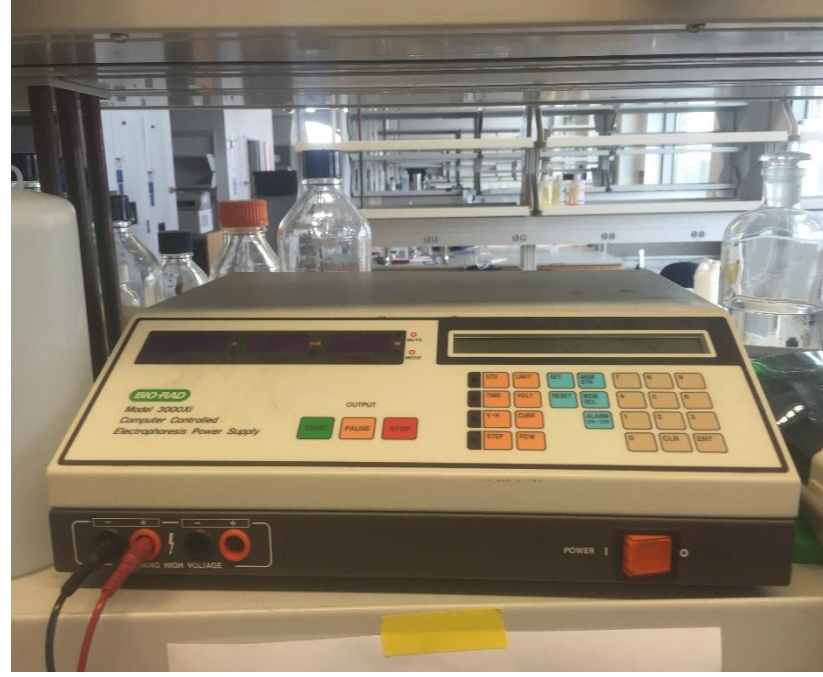
Figure 3. Gel running apparatus (Fisher Biotech FB-VE20-1, left) and high-voltage power supply (Bio-rad model 3000Xi, right).
