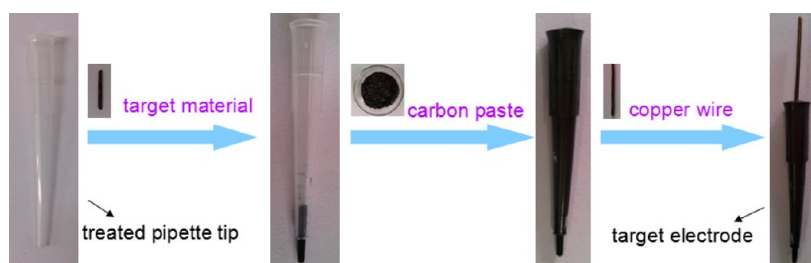
Figure 1. Schematic illustration of the fabrication of the integrated 3D-KSCs/inorganic nanocomposite electrode.
