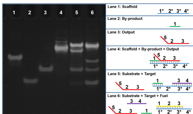
Figure 2. Native PAGE characterization of the DNA amplifier system. Lane 1: scaffold: 5 \mu\text{mol L}^{-1} \times 5 \mu\text{L} ; lane 2: byproduct: 5 \mu\text{mol L}^{-1} \times 5 \mu\text{L} ; lane 3: output: 5 \mu\text{mol L}^{-1} \times 5 \mu\text{L} ; lane 4: scaffold: 5 \mu\text{mol L}^{-1} \times 5 \mu\text{L} + byproduct: 50 \mu\text{mol L}^{-1} \times 0.5 \mu\text{L} + output: 50 \mu\text{mol L}^{-1} \times 0.5 \mu\text{L} ; lane 5: scaffold: 5 \mu\text{mol L}^{-1} \times 5 \mu\text{L} + byproduct: 50 \mu\text{mol L}^{-1} \times 0.5 \mu\text{L} + output: 50 \mu\text{mol L}^{-1} \times 0.5 \mu\text{L} + target: 0.5 \mu\text{mol L}^{-1} \times 0.5 \mu\text{L} ( 0.01 \times ); lane 6: scaffold: 5 \mu\text{mol L}^{-1} \times 5 \mu\text{L} + byproduct: 50 \mu\text{mol L}^{-1} \times 0.5 \mu\text{L} + output: 50 \mu\text{mol L}^{-1} \times 0.5 \mu\text{L} + target: 0.5 \mu\text{mol L}^{-1} \times 0.5 \mu\text{L} ( 0.01 \times ) + fuel: 50 \mu\text{mol L}^{-1} \times 0.5 \mu\text{L} . Reaction time = 2 h.
