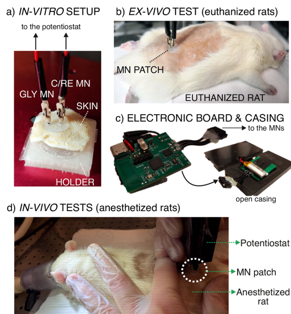
Figure 5. (a) Image of the in vitro setup, where a piece of rat skin is fixed in a holder to be analyzed with the MN biosensor. (b) Image of an on-body test using the MN GLY biosensor on a euthanized rat. (c) Image of the electronic board used for amperometric measurements, plus the casing used to introduce it and run the wireless data acquisition (KERIC). (d) Image of an in vivo test using the MN GLY biosensor in an anesthetized rat (UUBF).
