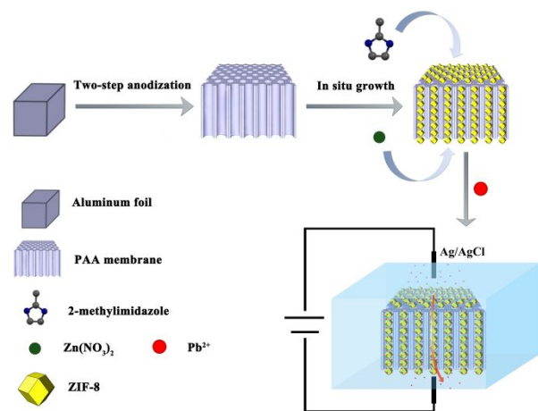
Scheme 1. Preparation of ZIF-8/PAA nanochannels composite membrane in situ growth and the biosensor prepared by the composite membrane was used to detect \text{Pb}^{2+} .
