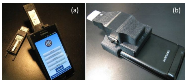
Figure 2. Attachment to cell phone used to read results from lateral flow assays. [Reproduced with permission from ref. 16. Copyright (2012) Royal Society of Chemistry.]
