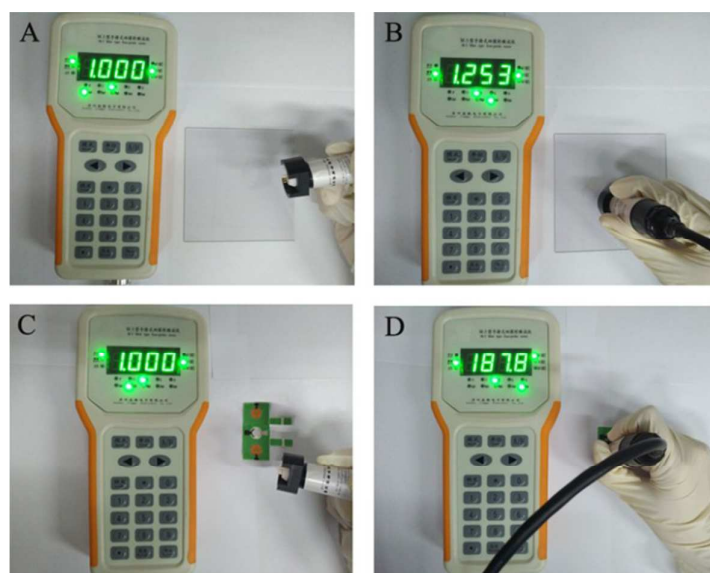
Figure 2. Four-probe tester is used to detect the resistance of ITO (A and B), and the Au-PWE (C and D), respectively.
