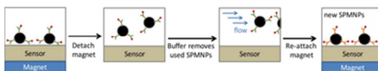
Figure 5. Re-usable SPMNP immunoassays. After analyte capture by both the antibody-coated SPMNPs, antigen bound SPMNPs are concentrated at the sensor surface by a magnet for signal detection. These are then released by detaching the external magnet and removed by flowing buffer solution. New SPMNPs are easily attached on the sensor surface by attaching the external magnet and ready for a new assay.
